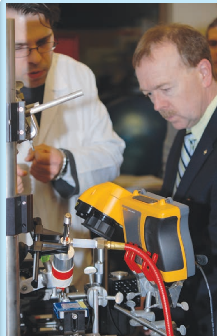
Hands on: Engineering research assistant Henry Lukic (left) explains the dynamometer—developed in the ADA Laboratories to test handpiece torque and power—to Dr. Ralph Howell of Suffolk, Va. Dr. Howell and others say the labs are a must-see when in Chicago. Story, Page 18.
