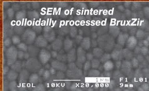
BruxZir's 50% smaller average grain size improves its physical properties.
