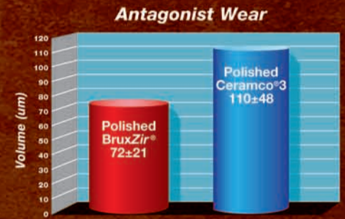
The antagonistic (Steatite balls) wear shows BruxZir only with 72±21 micron, which is significantly lower than Ceramco® 3 (110±48 micron). The University of Tübingen study was run using an eight chamber Willytec Chewing Simulator at 1.2 million cycles.
