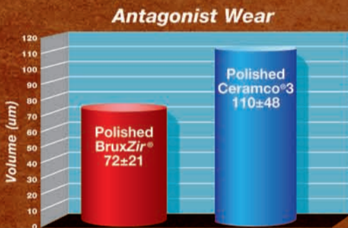
The antagonistic (Steatite balls) wear shows BruxZir only with 72±21 micron, which is significantly lower than Ceramco®3 (110±48 micron). The University of Tübingen study was run using an eight chamber Willytec Chewing Simulator at 1.2 million cycles.
