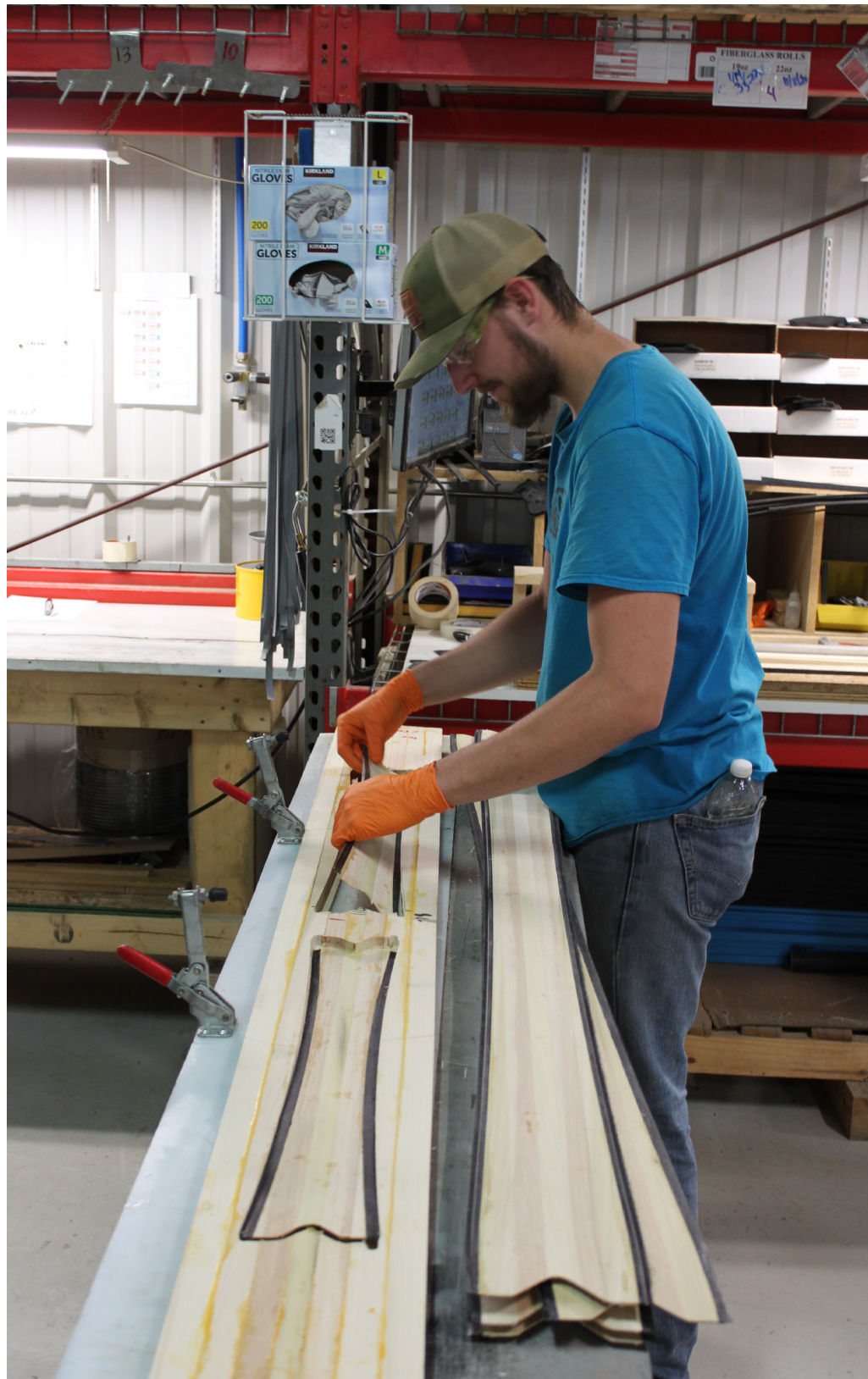
Shaggy's Zach Hardy crafts the core for a pair of custom skis.
