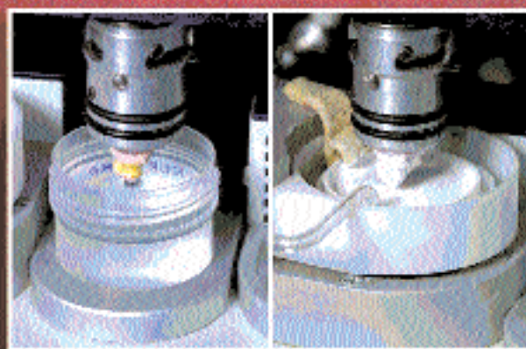
The outstanding fits and strength of these restorations are the result of an electronically deposited alumina oxide coping or bridge framework. This precise electro-deposition, made on the master die, results in marginal integrity that matches our best PFMs.
