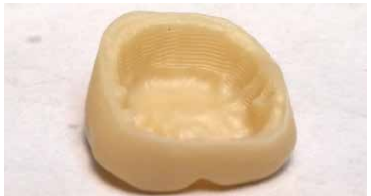
Figure 6: Circumferential retention groove technique creates a highly mechanical retentive surface.
