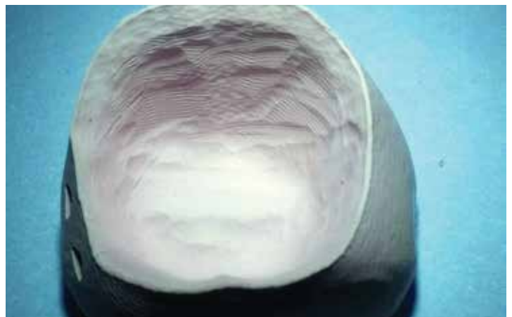
Figure 5: A technique of cutting circumferential retention grooves on the intaglio surface of milled zirconium before it is sintered.
